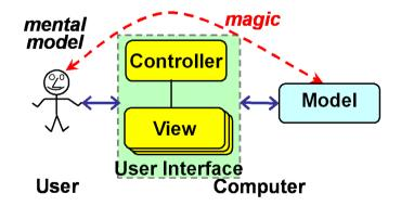
The Model is a representation of the user's information model. The *magic* in the above figure is that the user experiences the computer as an extension of their mind. The illusion is achieved by faithfully reflecting the user's mental model in the Model code. The user is in the driver's seat, and a View bridges the gap between their mind and the Model.
